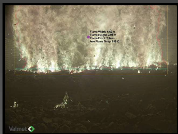
Grate visibility with flame profiling
